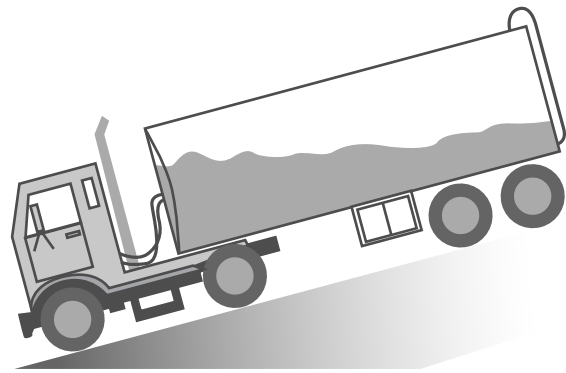
Figure 8-1: Smooth bore tank
